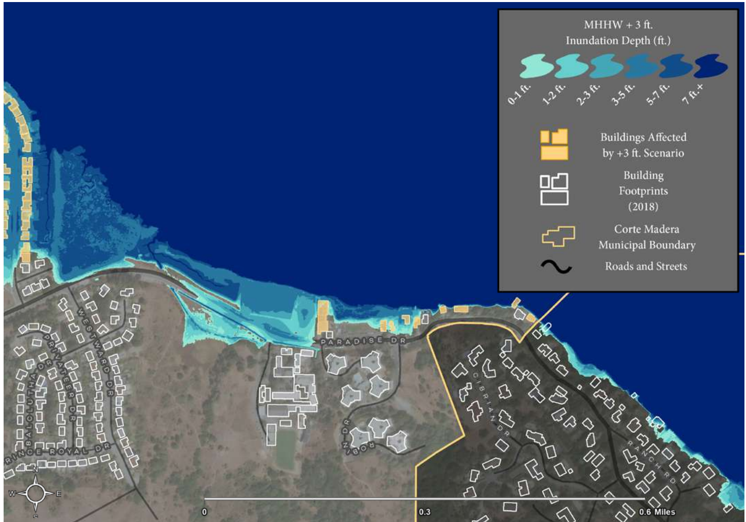
Figure 3.7. East Paradise Drive under a MHHW + 5.5 ft. scenario. Color shading depicts approximate depth of inundation. Mapping is based on 2019 LiDAR Data collected by Marin County and methodology can be found in Appendix D.
