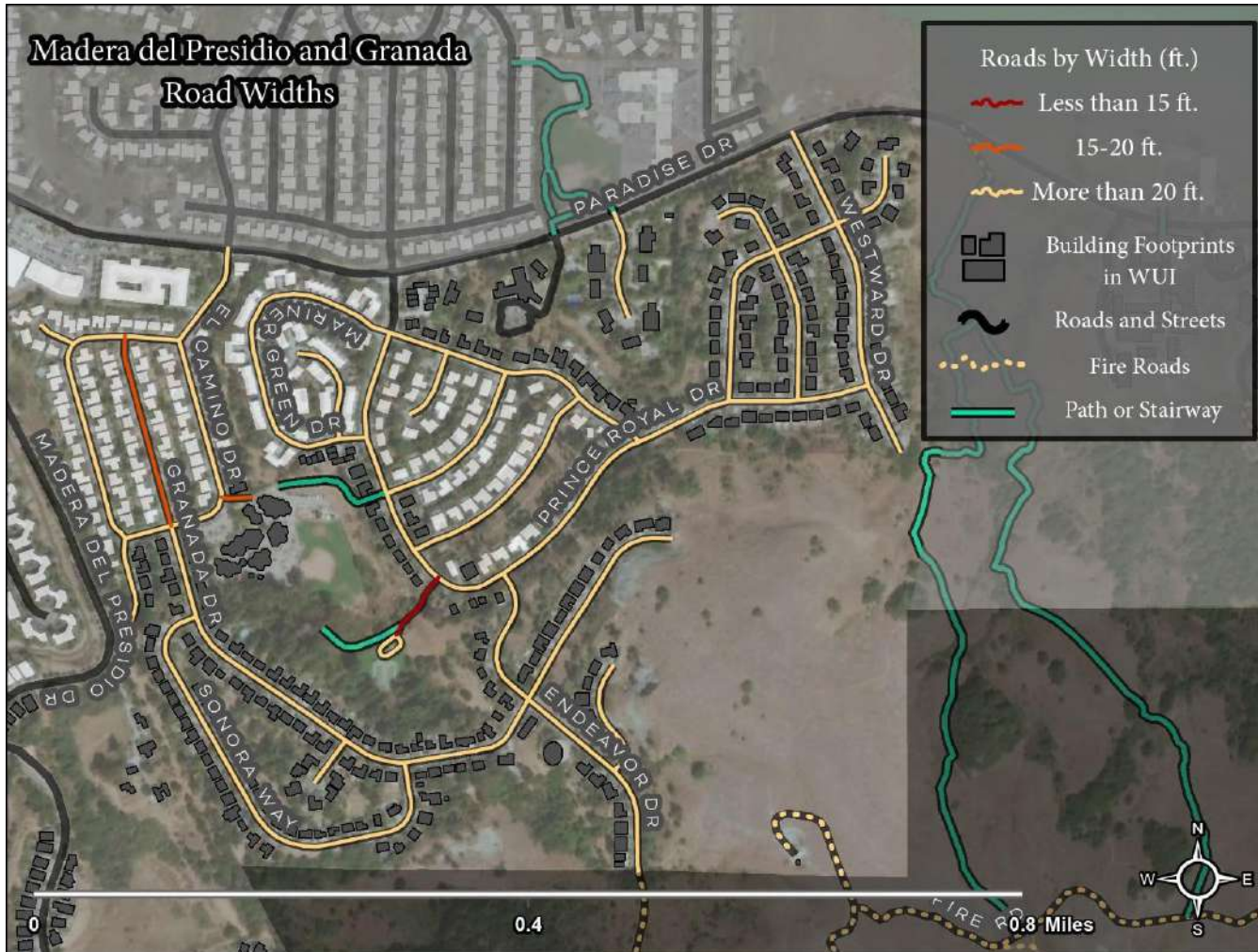
Figure 8 - Map depicting road widths in the Granada and Madera del Presidio neighborhoods, as ascertained by Nelson Nygaard field technicians. Although not as constricted as roads in other Hillside neighborhoods, careful coordination during a potential wildfire scenario in this area will be required, especially so as to avoid traffic jams as neighborhood streams empty onto Paradise Drive.
