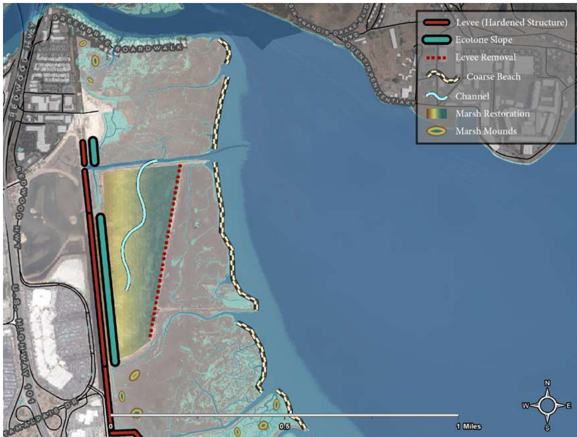
Figure 3.11. Conceptual design for potential restoration and adaptation options at Corte Madera Marsh and the railroad right-of-way.
