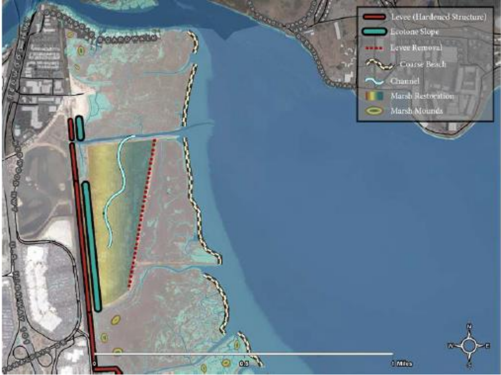
Figure 3.11. Conceptual design for potential restoration and adaptation options at Cortes Madera Marsh and the railroad right-of-way.
